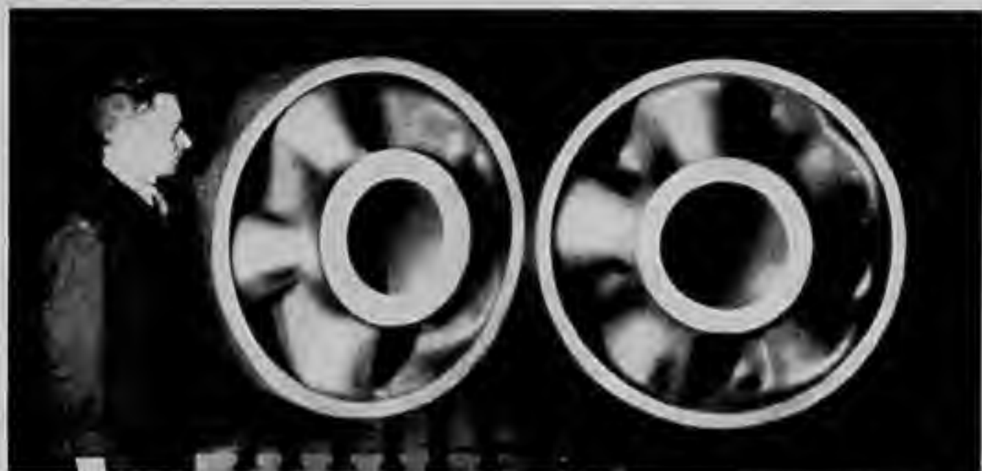
Fig. 6. Elektron magnesium alloy pulley castings, 35 in. diameter, as used on double-acting Bêche hammer. Castings of this type are made in weights up to 850 lbs.
